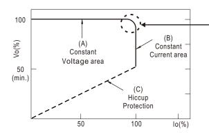
Typical output current normalized by rated current (%)
